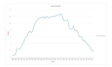
From this graph we can see that the power output in the morning from 8 AM to 10 AM is below 8 watt which is 60% output of total capacity of the solar plate.it is increasing as time increases after 10 AM the power output is fast increasing. Between the time 11 to 2 PM the output is between 10 to 12 Watt which is 100% and highest power output during a day after 2 PM it is decreasing as time passes and the power out-
