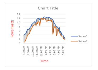
59 As we can see from above graph the power output of tracking system is much more than the power output of without tracking system. The change in the power output is high in the morning and evening time and it is normal at the afternoon time. So that's why we should use solar tracking systems for more gain of solar energy.by modifying this we can also do more in this to gain more and more energy
